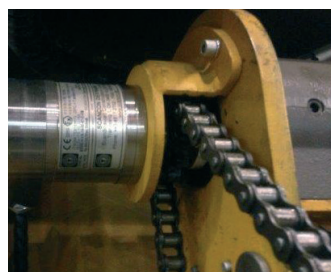
Cable drums on Mining conveyor belt vehicle. EXME absolute encoder.
