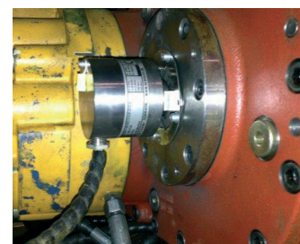
Mining drill machine and conveyor belt vehicle. REXM absolute encoder.
